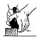
in complete contact with the wood. (The Illustration shows the correct way to hold the plane). When the rebate is "stopped", or does not go the full length of the work, the Cutter should be fitted in the forward position in the Plane Body. Very occasionally a rebate has to be worked on the opposite side of a wide piece of wood, and, in such a case, the Fence and Fence Arm should be transferred to the right hand side of the Plane. (Screwhole "M" on diagram).
